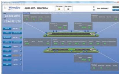
The **MET client** provides a geo-referenced overview of real time data from field sensors and external systems, allowing both the setting of alarms thresholds and a direct field sensors managements. Specific tools allow the compiling and emissions of aeronautical and synoptic weather reports, both in a manned and unmanned way. A historical archive for browsing and managing meteorological data is also available.
